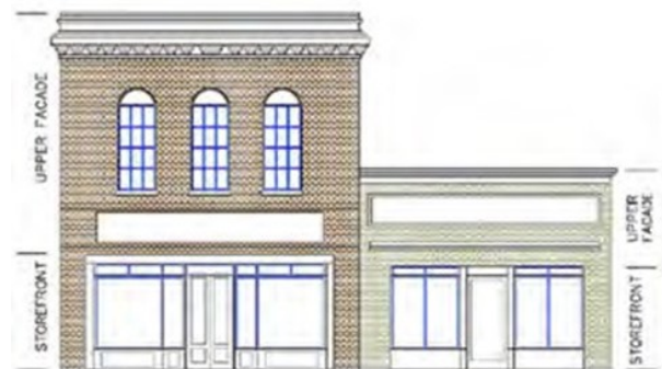
Elements of the commercial façade.
